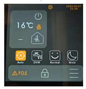
**F05** is one of the most common fault codes and means that the water is not moving quickly enough around the system. This could be because the filters are dirty, there is air in the system or there is not enough water pressure. Have you recently bled the radiators? If so, this could be the cause of the fault code appearing, and you must top up the pressure in the system. Check all of the above and restart the unit to see if the fault code has disappeared.
