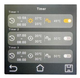
Each timer can have heating or hot water or both. In the above example, note the top timer is active and so is orange (use the slider to activate/deactivate it) and is for both heating and hot water.
