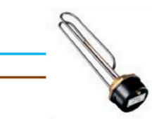
Immersion heater L to 20 and N to 21 in cylinder, but ONLY if under 2000 Watts.
